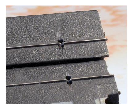
Strip a couple of inches of insulation from the end of the wire and feed the end up through the bottom of the track. Make a U bend in the wire and feed the end of that down through the hole on the other end of the notch.
